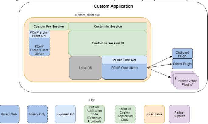
\*Partner Virtual Channel Plugins can be developed using the Virtual Channel SDK, to enable this you can combine the PCoIP Client SDK with the PCoIP Virtual Channel SDK.
